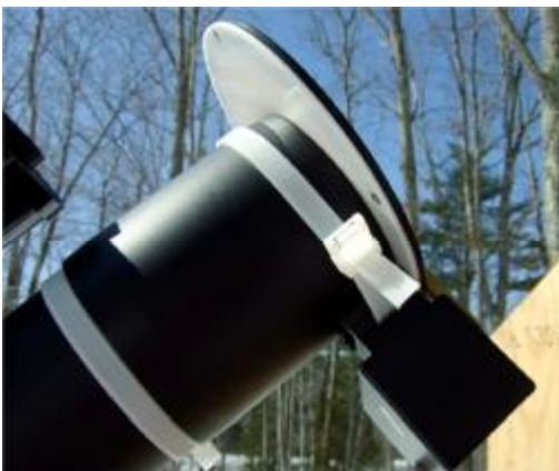
Figure 2. The Flip-Flat mounted to a retractable dew shield. Note the additional zip tie below the dew shield to keep it from sliding down.
