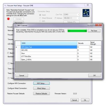
For nearly all modern routers, the Security Type will be "WPA With Passphrase". Click Apply New Settings and allow a few minutes for the local WiFi DHCP server to assign a new IP address to the Optec WiFi board.
