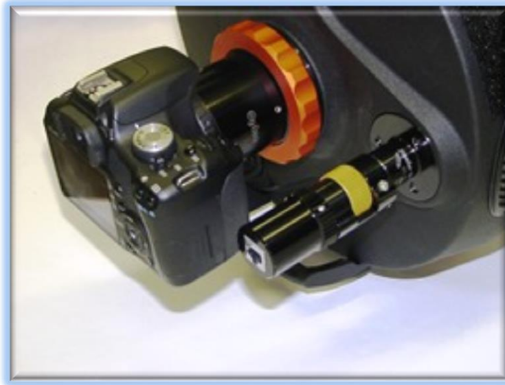
FocusLynx QuickSync motor with Feather Touch FTM Micro Pinion Retro-fit on a Celestron C11 HD.
