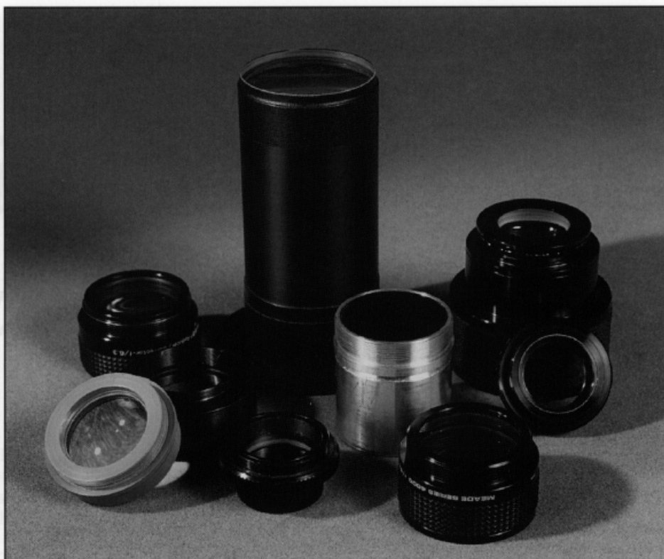
Focal reducers come in all shapes and sizes. The author feels they are one of the most important accessories for digital imaging since they are ideal for adjusting a telescope's effective focal length to a CCD's pixel size.
