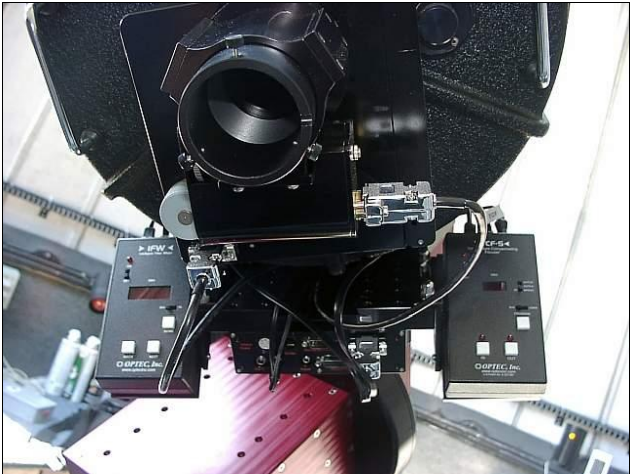
TCF-S Focuser and IFW Filter Wheel mounted to the Paramount ME using Optec's Paramount ME Mounting & Wiring Kit.
